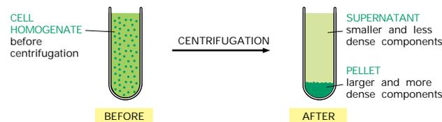
Centrifugation is the most widely used procedure to separate a homogenate into different parts, or fractions. The homogenate is placed in test tubes and rotated at high speed in a centrifuge (sometimes called an ultracentrifuge). Present-day ultracentrifuges rotate at speeds up to 100,000 revolutions per minute and create enormous forces, as high as 600,000 times gravity.
